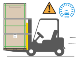
Control the speed to prevent tipping.
